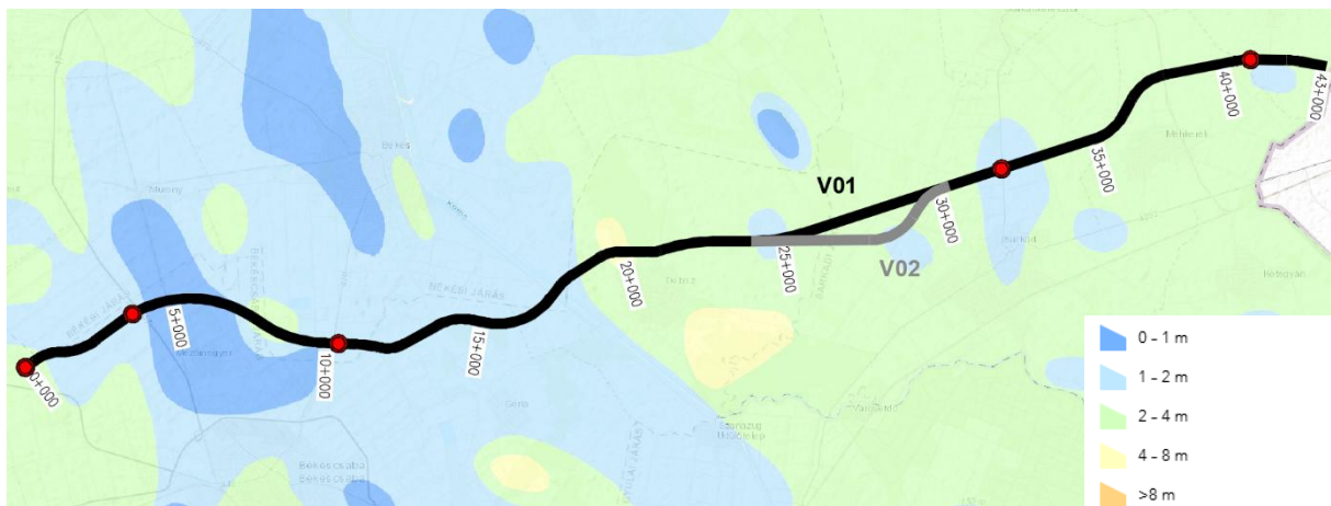
Figure 8. Groundwater surface rest level below the surface in the vicinity of the trail
