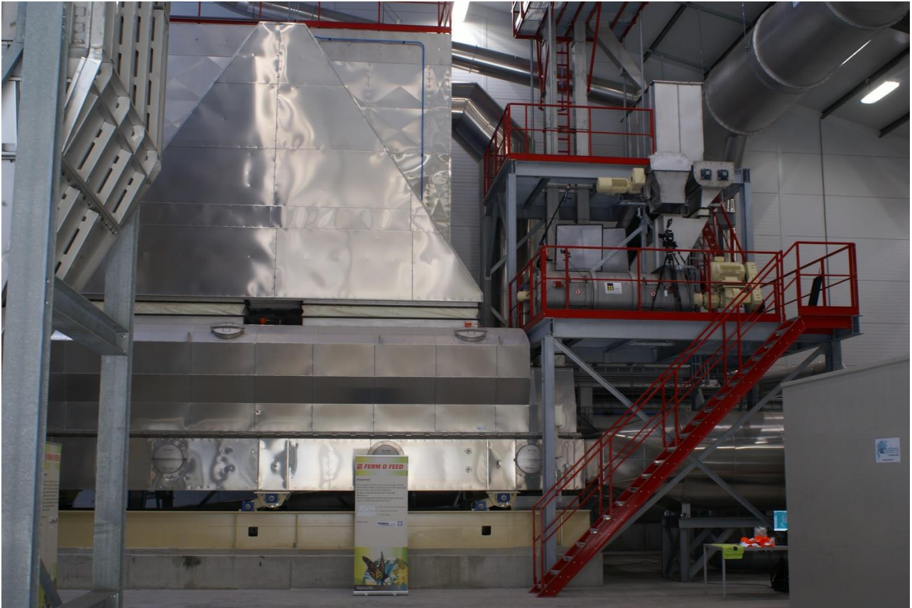
Fluid bed dryer for chicken manure
